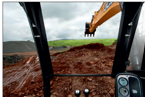
High all around visibility aided by roof mounted glass for working at height
