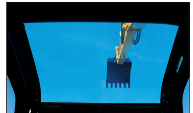
High all around visibility aided by roof mounted glass for working at height
