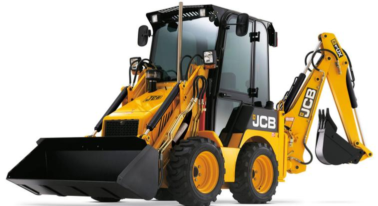
The launch of the ICX skid-steer has allowed the manufacturer to also stake its claim to developing the world's smallest backhoe loader, providing excavation and skid-steer performance in a single package.
